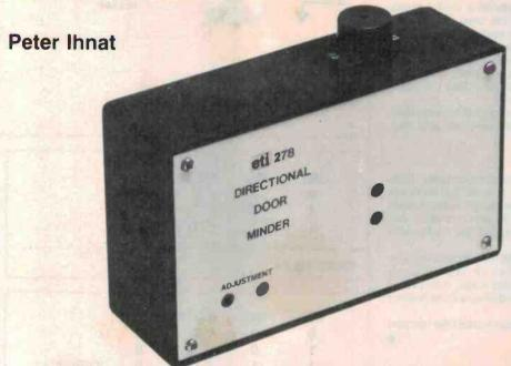
Most electronic door minders function by having a beam of light shining across a doorway interrupted, but are incapable of detecting whether the light beam is broken by a person entering or leaving the room. This project overcomes that problem with the aid of digital logic.
