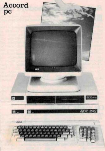
The Accord ACC-8000 computer is a newcomer to the Australian market. It is a Z80-based computer that runs under the improved CP/M operating system (CP/M 3.0). This optimises the use of the machines 128K memory, and its 'hashed' directory structures speed up the loading of programs and data. The optional hard disk (10, 20 and 40 M) is also a networking node which allows an ACC-8000 to become a file server and print spooler for up to 255 other computers.
