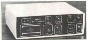
Hey, good lookin'! The ETI lab (thanks to Geoff Nicholls) housed the project in a good looking plastic case. The inputs and outputs are all on the rear. Note the bargraph tuning indicators. The RFE indicator shows when corrupt copy is being received.
